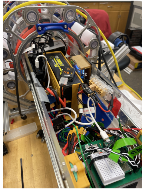
Fig. 4: Internal retractable electronic drawer of the sub
